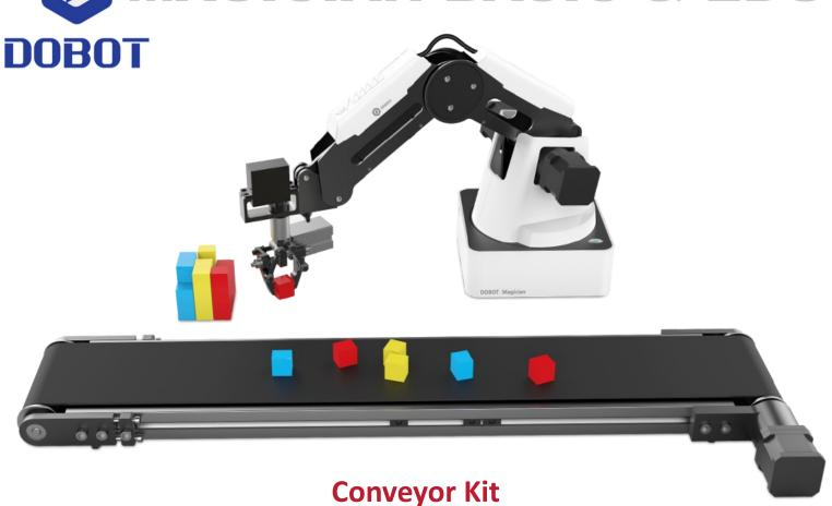
The Conveyor Kit for DOBOT Magician makes it possible to own a complete simulated production line. The powerful and programmable DOBOT Magician, when combined with conveyor belt of adjustable speed, distance and color sensor, is the ideal and perfect tool for you to create a highly effective simulated production line, or even to apply to actual factory
