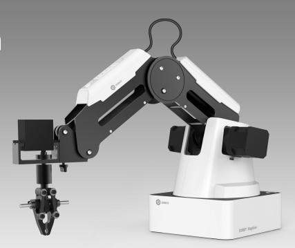
DOBOT Magician is a multifunctional desktop robotic arm for practical training education. Installed with different end-tools, DOBOT Magician can realize interesting functions such as 3D printing, laser engraving, writing and drawing. It supports secondary development by 13 extensible interfaces and over 20 programming languages, which really makes your creativity and imagination increase without any limitation.
